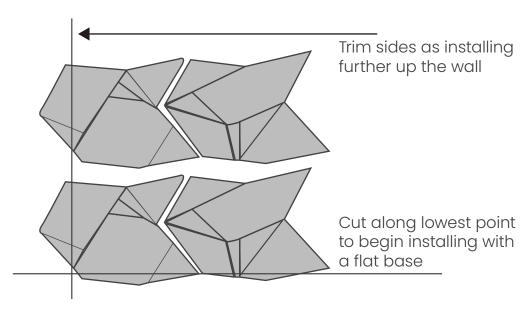
**Installing with Dry Joint:** Take time once the pattern is laid to cut thin stones to fill small gaps between the larger joints. This is very important, it will break up the pattern and provide the perfect hand crafted stone masonry look.
